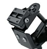
The functional bracket for the navigation systems and the smartphone cradle from BMW Motorrad is securely attached to the handlebar clamp. This ensures that it can be positioned in the rider's direct field of vision. In addition, the bracket complements perfectly the cockpit area.
