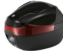
With a volume of 29 litres, the light topcase offers enough space for a helmet and convinces in everyday life as well as on short tours. The black plastic topcase is lockable, has a large reflector on the rear side and a BMW badge on the lid. The maximum payload is 3 kg.
